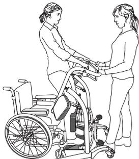
QuickMove can be used to train the patient's standing, sitting and sit-to-stand function. To measure improvement, use a stopwatch or clock with a second hand to time the patient.
